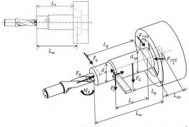
$F_G/[N]$  = workpiece mass / [kg] x 9,81 / [m/s<sup>2</sup>]
