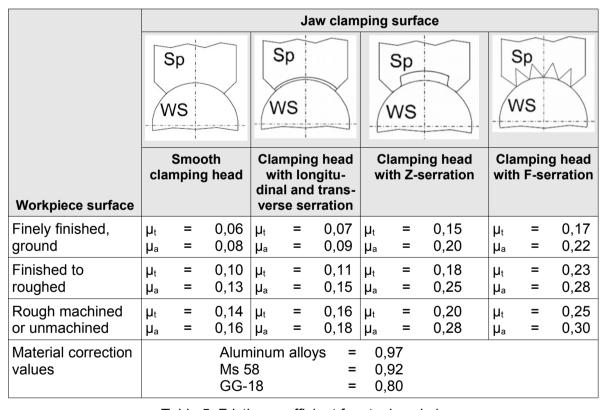
Table 5: Friction coefficient for steel workpieces
