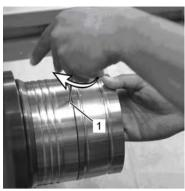
5. Tighten all clamping screws of the base end-stop in the spindle flange clockwise with an allen wrench. The base end-stop is now secured.
