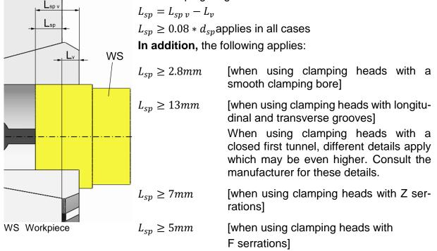
If HAINBUCH uses a different and shorter clamping length in this clamping situation drawing, this will have been checked against the specific parameters for this type of application and found to be sufficient.
