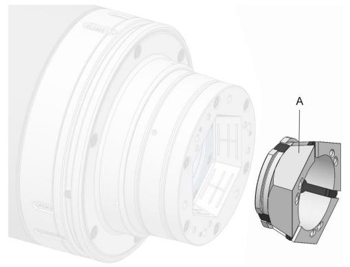
A Clamping head [clamping element]
