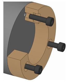
1. Unfasten and remove the fixing screws on the changing part.
