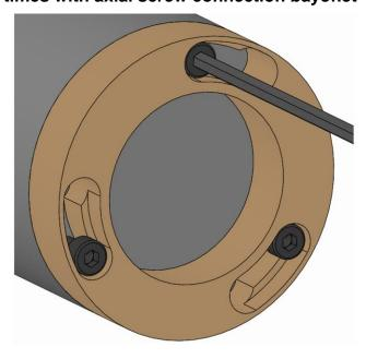
1. Unfasten the fixing screws on the changing body a few turns without removing them.
