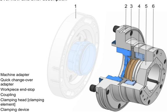
The clamping device can be used as a through-chuck for machining bar stock and also as an end-stop chuck.
