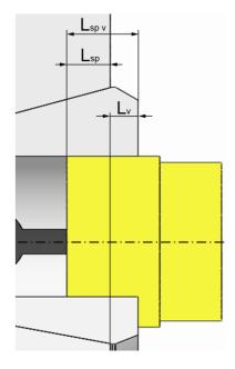
Without exception, never go below the total clamping length  $L_{sp v}$  of the workpiece, which measures at least 7 mm.
