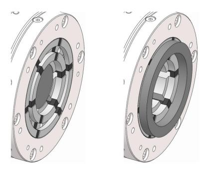
5. Release tension on the dressing pin / dressing ring. To do this, if necessary secure the dressing pin / dressing ring to prevent it from falling out.
