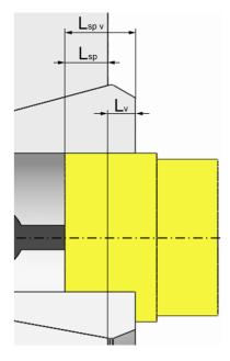
Without exception, never go below the total clamping length  $L_{sp v}$  of the workpiece, which measures at least 3 mm.
