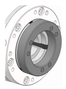
Release tension on the dressing pin / dressing ring. To do this, if necessary secure the dressing pin / dressing ring to prevent it from falling out.
