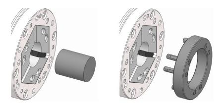
Install the dressing pin in the clamping device to prevent it from getting damaged when the HSW clamping head is getting machined. And/or, install the dressing firmly home in the HSW clamping head, aligning the pins in the dressing ring with the alternating bores in the HSW clamping head.
