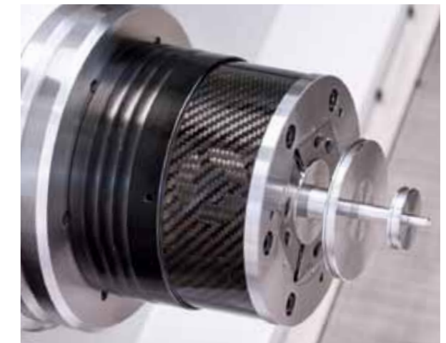
Sample application of the new TOPlus lightweight chuck for machining a shaft.
