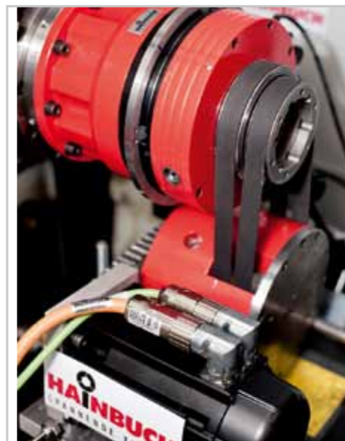
Electric hollow vise and servomotor
