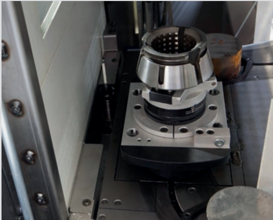
Stocking and changing station on the workpiece feeder belt to change-over the clamping head.
