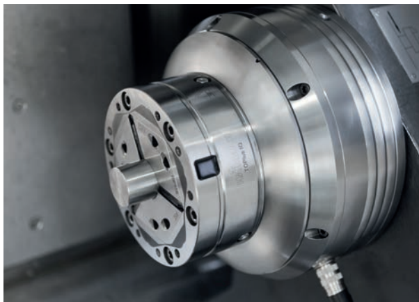
Chuck with cable: The TOPlus IQ is an intelligent data supplier for Industry 4.0.
