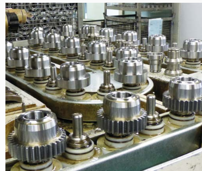
▲ The automatic loading system with the gears on the Gleason Pfauter machine.
