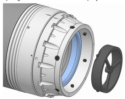
6. Install the mounting aid in the functional unit to enable the mounting aid to engage in the grooves of the drawtube adapter in the functional unit.
