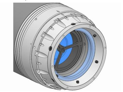
6. Using the mounting aid, screw the drawtube adapter of the functional unit firmly home on the machine drawtube.
