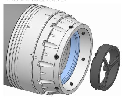
5. Install the mounting aid in the functional unit to enable the mounting aid to engage in the grooves of the drawtube adapter in the functional unit.
