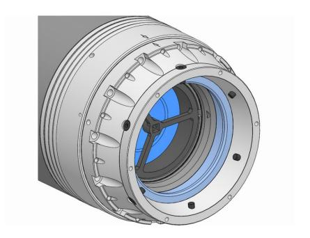
7. Using the mounting aid, unscrew and remove the drawtube adapter on the functional unit from the machine drawtube.
