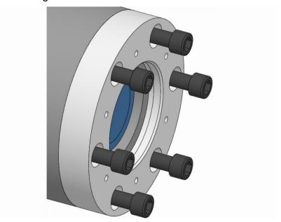
4. Screw in the spindle flange fixing screws and tighten them gently.
