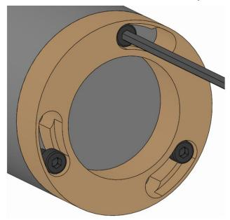
1. Unfasten the fixing screws on the changing body a few turns without removing them.
