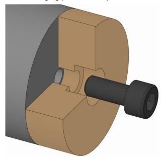
2. Screw in the changing part fixing screw and tighten it to the specified tightening torque [see »Screw tightening torques « chapter].
