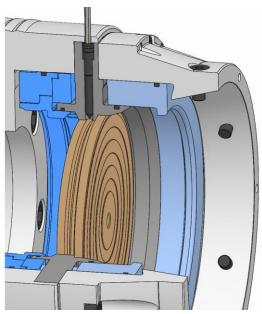
Unscrew the clamping screws from the base end-stop until the base end-stop can be lifted out.
