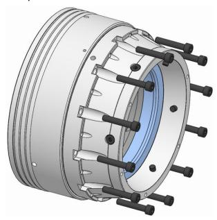
4. Unfasten and remove the fixing screws on the functional unit.
