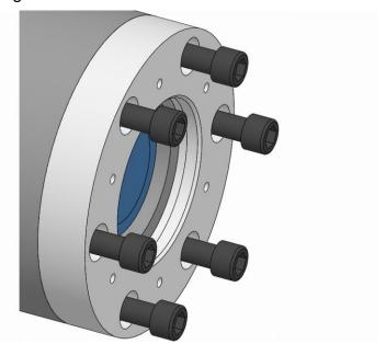
Screw in the changing part fixing screws on the spindle flange and tighten to the specified tightening torque [see »Screw tightening torques« chapter].
