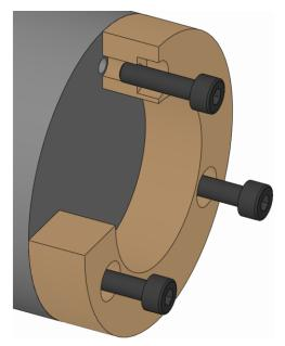
Unfasten and remove the fixing screws on the changing part.
