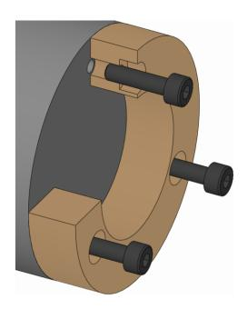
2. Screw in the changing part fixing screws on the changing part and tighten to the specified tightening torque [see »Screw tightening torques « chapter].
