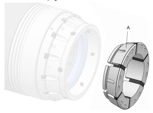
A Clamping head [clamping element]
