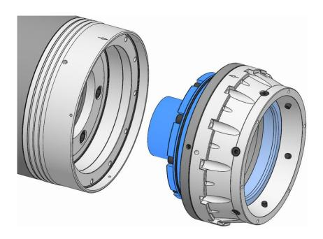
Take down the functional unit from the spindle flange.
