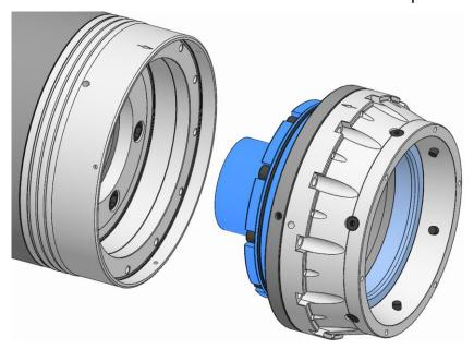
4. Fit the functional unit on the spindle flange until the balancing marks on the spindle flange are aligned with those on the functional unit.
