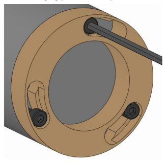
Screw in the changing part fixing screws and tighten to the specified tightening torque [see »Screw tightening 3. torques« chapter].
