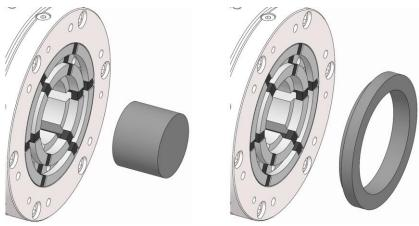
6. Remove the dressing pin from the clamping device. And/or remove the dressing ring from the HSW clamping head.
