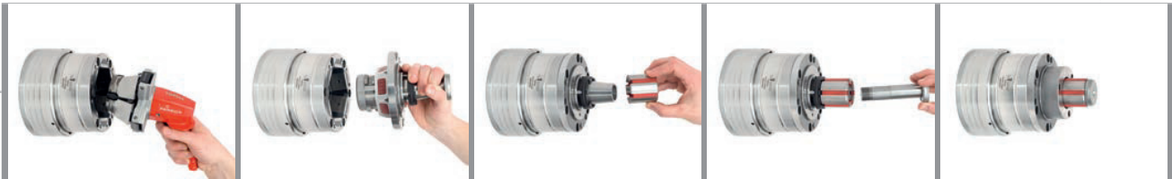
Remove clamping head Insert MANDO Adapt T211 Fit on segmented clamping bushing Screw in draw bolt Clamping device set-up
