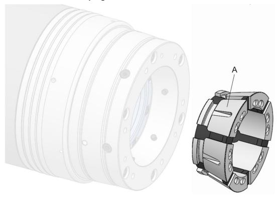
A Clamping head [clamping element]
