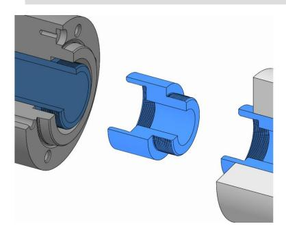
Screw the drawtube adapter into the functional unit using its thread or screw it to the machine drawtube and tighten it down.
