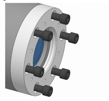
Screw in the changing part fixing screws on the spindle flange and tighten to the specified tightening torque [see »Screw tightening torques « chapter].
