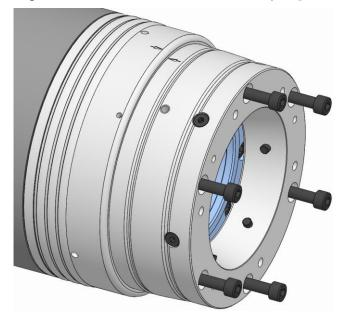
7. Screw in the fixing screws on the functional unit and tighten them gently.
