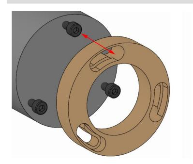
1. Place the changing part on the product so that the screw head on the changing part fixing screw fits through the bayonet opening.
