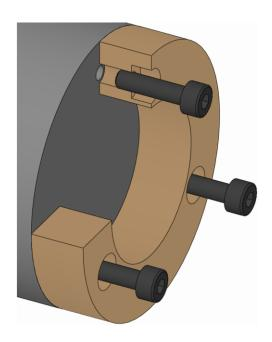
2. Screw in the changing part fixing screws on the changing part and tighten to the specified tightening torque [see »Screw tightening torques « chapter].
