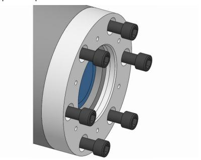
3. Unfasten and remove the fixing screws on the spindle flange.
