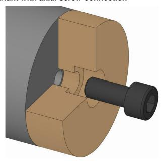
1. Unfasten and remove the fixing screw on the changing part.
