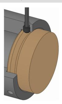
Unscrew the clamping screws from the changing part until the changing part can be lifted out.
