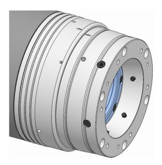
Turn back the functional unit until the balancing marks on the spindle flange are aligned with those on the functional unit.
