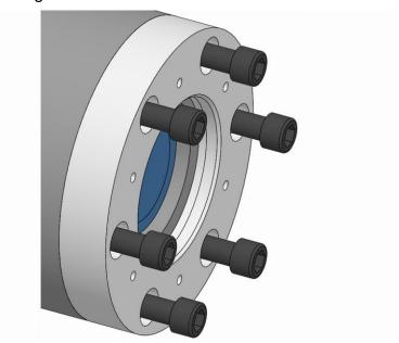
Screw in the spindle flange fixing screws and tighten them gently.
