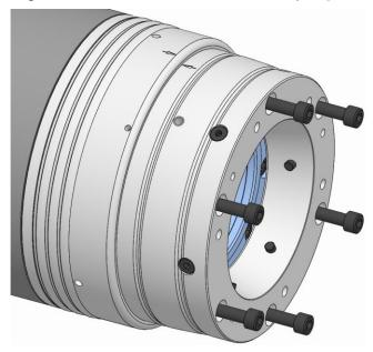
7. Screw in the fixing screws on the functional unit and tighten to the specified tightening torque [see »Screw tightening torques« chapter].
