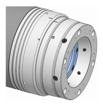
5. Turn back the functional unit until the balancing marks on the spindle flange are aligned with those on the functional unit.
