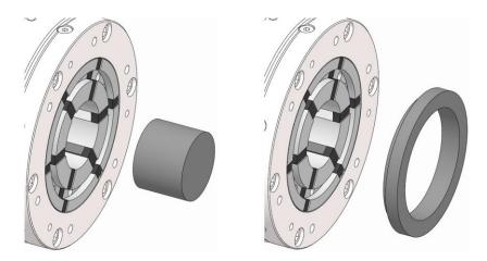
2. Install the dressing pin in the clamping device to prevent it from getting damaged when the HSW clamping head is getting machined. and/or, install the dressing ring firmly home in the turned groove in the HSW clamping head.
