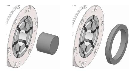
2. Install the dressing pin in the clamping device to prevent it from getting damaged when the HSW clamping head is getting machined. and/or, install the dressing ring firmly home in the turned groove in the HSW clamping head.
