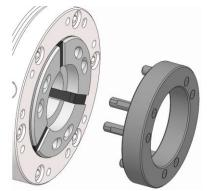
6. Remove the dressing pin from the clamping device. And/or remove the dressing ring from the HSW clamping head.
