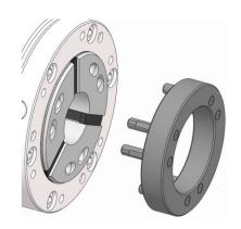
Install the dressing pin in the clamping device to prevent it from getting damaged when the HSW clamping head is getting machined. And/or, install the dressing firmly home in the HSW clamping head, aligning the pins in the dressing ring with the alternating bores in the HSW clamping head.
