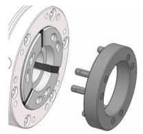
6. Remove the dressing pin from the clamping device. And/or remove the dressing ring from the HSW clamping head.
