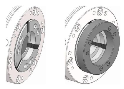
5. Release tension on the dressing pin / dressing ring. To do this, if necessary secure the dressing pin / dressing ring to prevent it from falling out.
