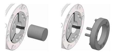
2. Install the dressing pin in the clamping device to prevent it from getting damaged when the HSW clamping head is getting machined. And/or, install the dressing firmly home in the HSW clamping head, aligning the pins in the dressing ring with the alternating bores in the HSW clamping head.
