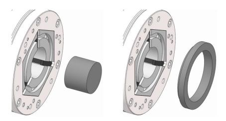
Install the dressing pin in the clamping device to prevent it from getting damaged when the HSW clamping head is getting machined. and/or, install the dressing ring firmly home in the turned groove in the HSW clamping head.
