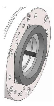
5. Release tension on the dressing pin / dressing ring. To do this, if necessary secure the dressing pin / dressing ring to prevent it from falling out.
