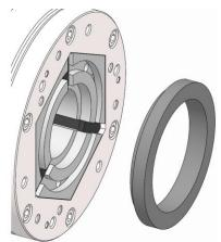
6. Remove the dressing pin from the clamping device. And/or remove the dressing ring from the HSW clamping head.
