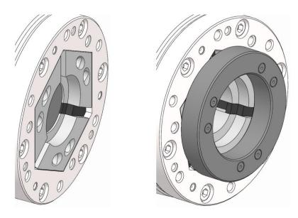
5. Release tension on the dressing pin / dressing ring. To do this, if necessary secure the dressing pin / dressing ring to prevent it from falling out.
