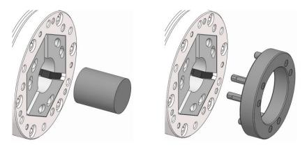
2. Install the dressing pin in the clamping device to prevent it from getting damaged when the HSW clamping head is getting machined. And/or, install the dressing firmly home in the HSW clamping head, aligning the pins in the dressing ring with the alternating bores in the HSW clamping head.
