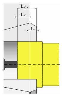
Without exception, never go below the total clamping length  $L_{sp v}$  of the workpiece, which measures at least 6 mm.
