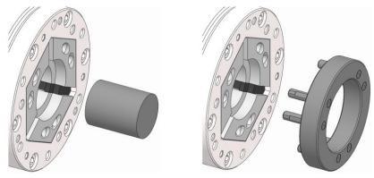
6. Remove the dressing pin from the clamping device. And/or remove the dressing ring from the HSW clamping head.
