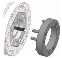
Remove the dressing pin from the clamping device.
