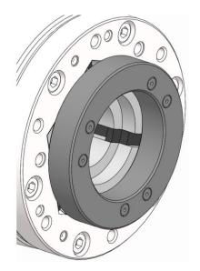
5. Release tension on the dressing pin / dressing ring. To do this, if necessary secure the dressing pin / dressing ring to prevent it from falling out.
